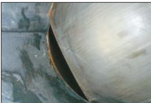
Interface Between Rubber Liner & Carbide Coated Ball
