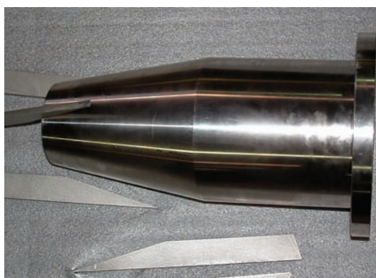
Pictured left: is a 10-inch diameter, de-coke t-section. The overlay is 200 degree grid, .350 thick.
