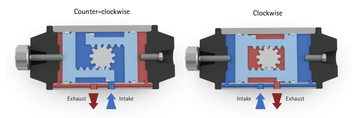
Counter clockwise output operation is achieved by inserting pressure into the intake to force the pistons apart thus rotating the actuator pinion counter clockwise. During the operation, air from the outer chambers is exhausted. Clockwise output operation is achieved by reverse of the above.
