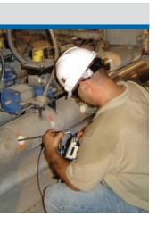
Unlike other testing methods that require the removal of large amounts of insulation, ValvTechnologies requires only small drill holes for access with a 3/8 inch diameter transducer.
