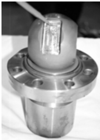
8) Remove ball, after marking orientation and protect from possible damage.
