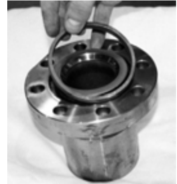
6) Remove body seal or gasket, depending upon valve design
