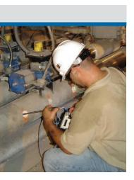
Unlike other testing methods that require the removal of large amounts of insulation, ValvTechnologies requires only small drill holes for access with a 3/8" diameter transducer.
