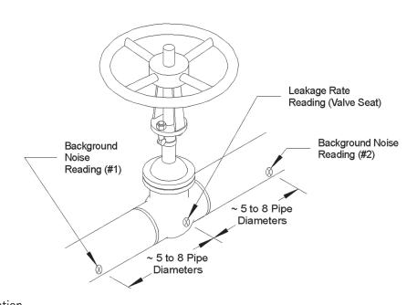
The underlying theory is simple: a leaking isolation valve is releasing energy and the ultrasonic emissions or noise levels coming from that valve can proxy the rate of energy release (i.e. the flow rate). ValvTechnologies takes that premise to the next level and beyond. Using knowledge-based software, ValvTechnologies is able to correlate the noise or ultrasonic emissions from a subject valve to a vast database of valves with known, laboratory verified leakage rates.
