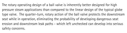
ValvTechnologies expanded upon the strengths of the ball valve by incorporating proprietary design features that extend the life of the standard, rotary design. Core to the design is the integral seat. As part of valve end cap, and positioned away from the flow path, leak paths and interference from particulates are eliminated.
